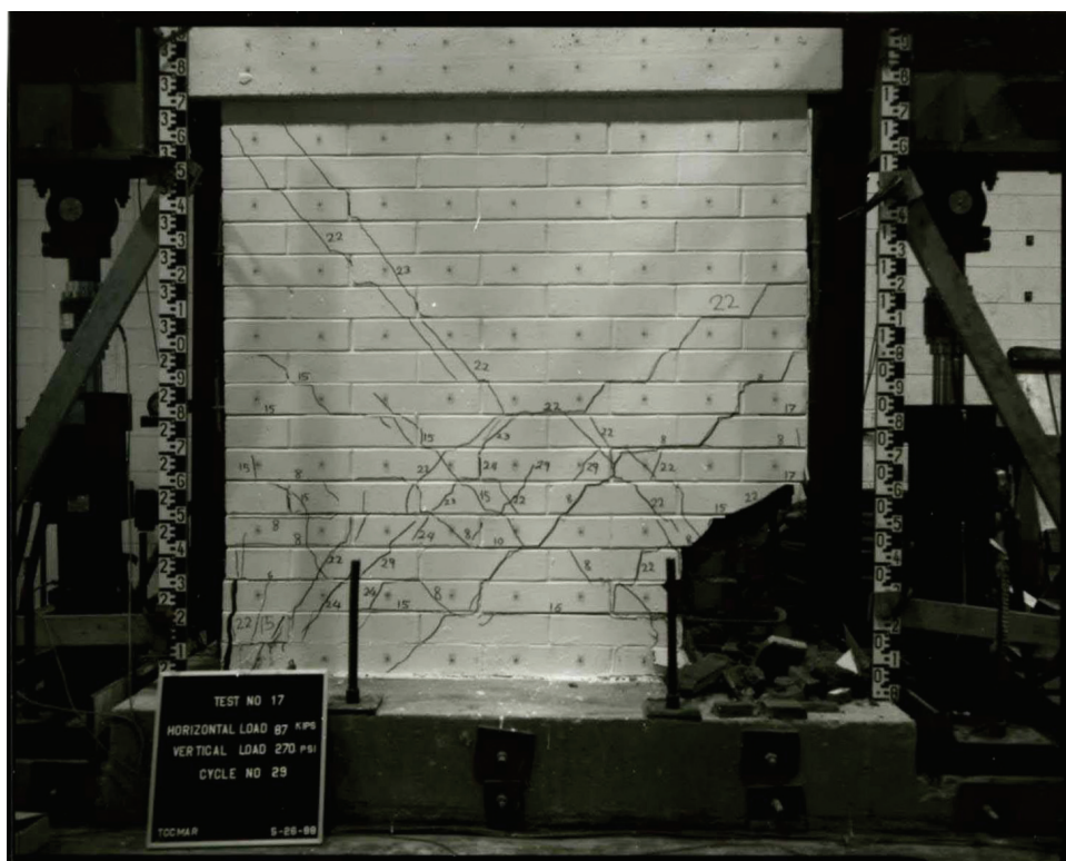
Figure 5 – Cracking and Crushing of Specimen 17 right after 20% Load Drop (Shing et al. 1991)
